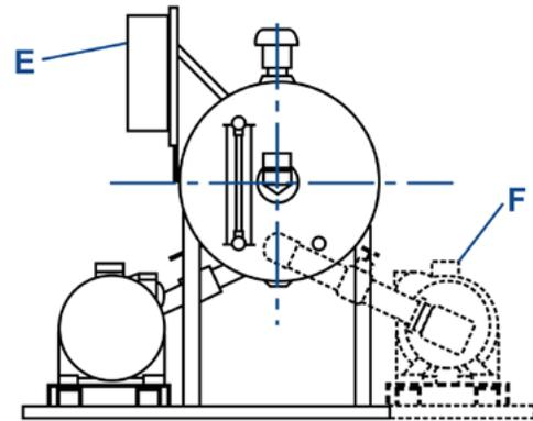
(A) Roth patented one foot NPSH pump guaranteed to pump boiling water with only one foot suction head in capacities up to 190 GPM. Liquid end and mechanical end are separated by a mechanical seal. Shaft is supported by two ball bearings. No water lubricated bearings required.
